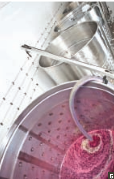
The winemaking process: 1) Hand-picked grapes. 2) Grapes being poured into a de-stemmer/crusher. 3) A stainless steel auger crushes grapes and removes stems. 4) Grapes being pressed. 5) Crushed grapes being pumped into fermenter. 6) Solution made of dry yeast and water ready to be pumped into a large stainless steel tank containing fermenting wine. 7) Monitoring the fermentation process. 8) The bottling line.
