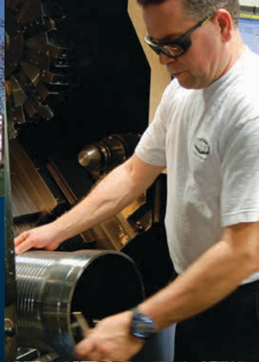
Machining King Combination Nipples in Chestertown
